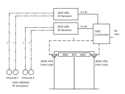
Operation: Doors normally closed, not latched. Two 8310-3856Ws actuators to independently signal each door to swing.
