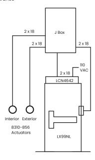
Operation: When panic device is mechanically dogged both interior and exterior actuators will be enabled through LX switch. When device is undogged actuators will not function.
