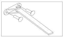
2. For pull systems, slide the pull arm roller into the track, then insert a track cap on each end of the track and attach the track to the door:
