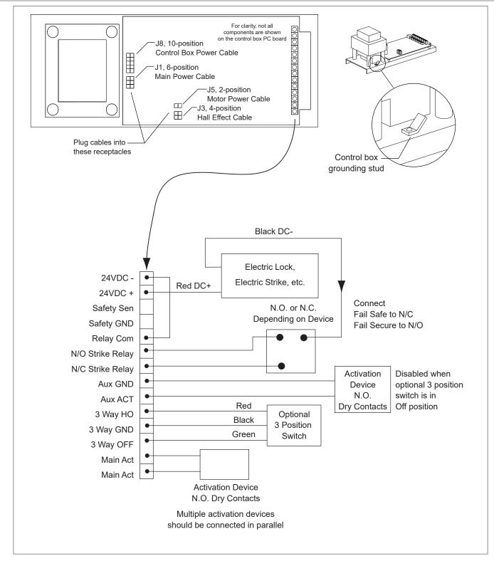
Connection to external devices must be made using CL2, CL2P, CL2R, or CL2X Class 2 wire or equivalent.
