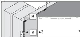
3 Remove template, and drill holes where marked with a 1/8" drill bit.
