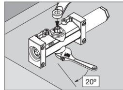
7 Install PA Shoe to frame, then shoe the rod & shoe.
